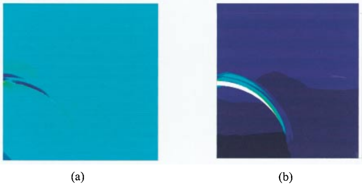
Figure 6. Contours of radial stress over the deformed unit cell configuration, (a) on the debonding initiation, and (b) on fracture propagation.
